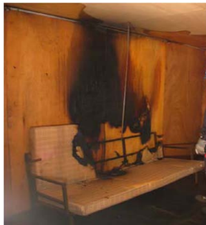
Fire extinguished by water based system in standard laboratory test
